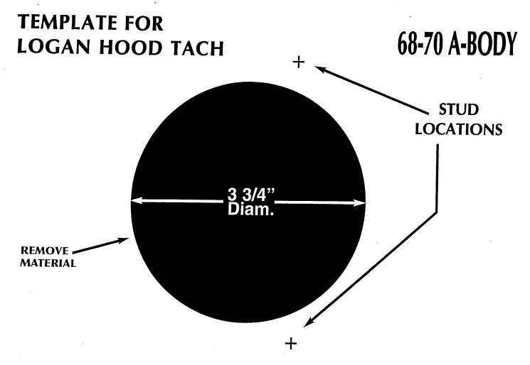
Carefully attach the template to the hood with tape in the indicated position (2 Inches from the driver's side of the hood and 12 Inches forward of the rear corner). Mark and carefully remove metal from the darkened areas.
