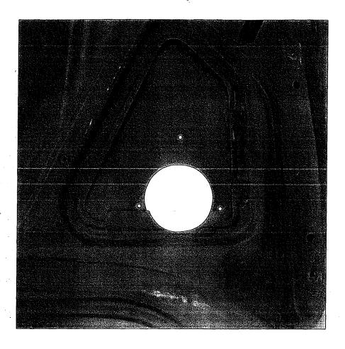
**NOTE**: THIS TACH TEMPLATE RESEMBLES ORIGINAL CUTTING DIMENSIONS. YOU WILL NEED TO REMOVE A PORTION OF THE UNDER HOOD BRACING AT THE DRIVERS SIDE REAR OF HOOD. (SEE IMAGE)
